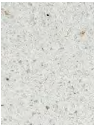
PRECAST OFF WHITE CON- CRETE TO COLLONADE -SHOT BLAST FINISH WITH QUARTZ AGGREGATE
